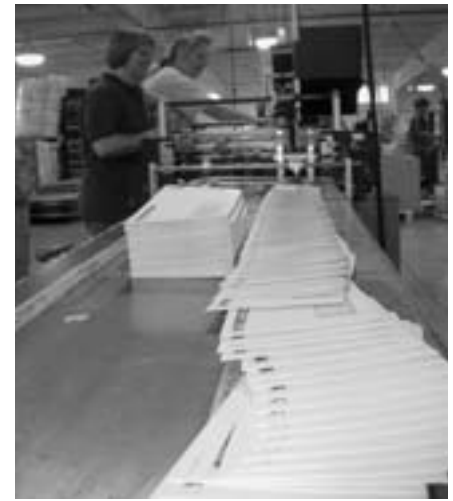
Address quality is important for improving mail deliverability. Inkjet systems at A.M. Mailing Services, Inc. print addresses that USPS automated equipment can easily scan.
